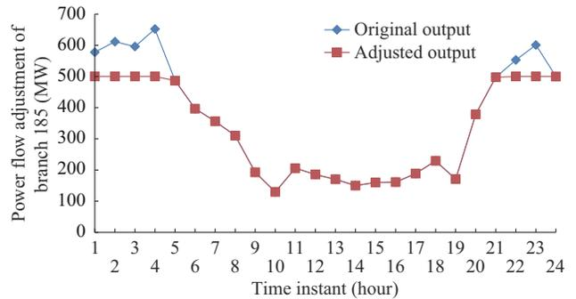
Fig. 5. Power flow adjustment of branch 185 caused by maintenance of branch 186 on the 30<sup>th</sup> day.
