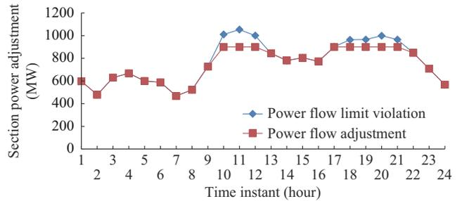
Fig. 4. Section power adjustment caused by maintenance of branches 98 and 99 on the 28<sup>th</sup> day.
