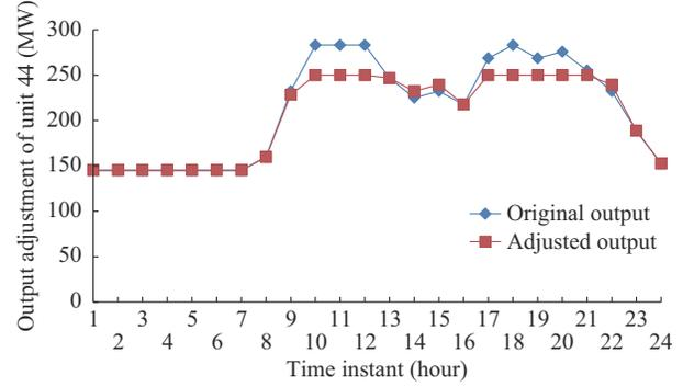
Fig. 3. Output adjustment of unit 44 caused by maintenance of branches 153 and 159 on the first day.
