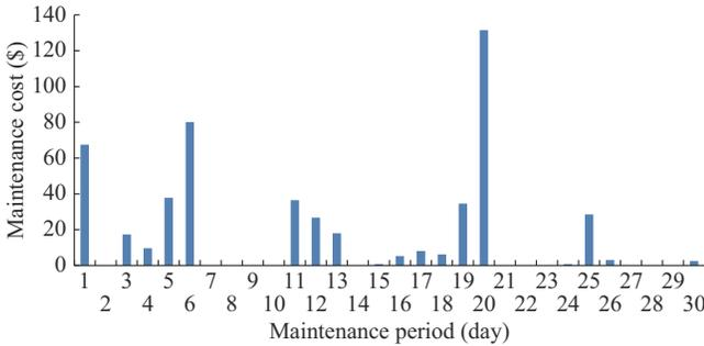
Fig. 2. Influence of branch 153 on increase in MOC during maintenance on different days.
