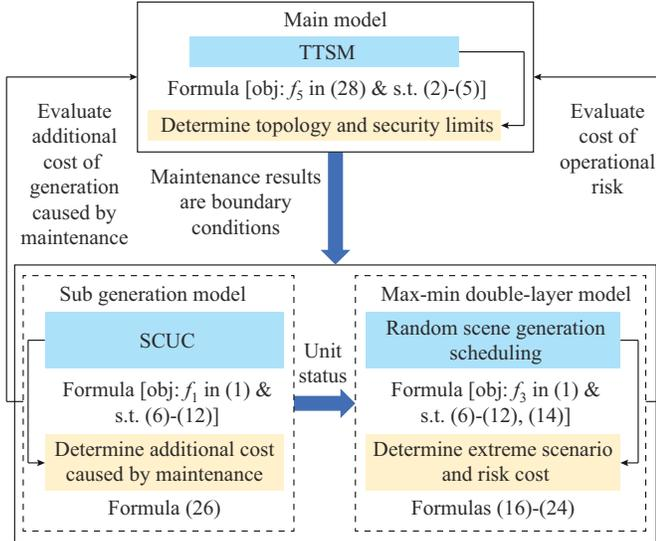
Fig. 1. Schematic of model structure.
