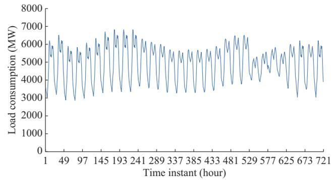
Fig. A2. Monthly load forecasting in each hour.
