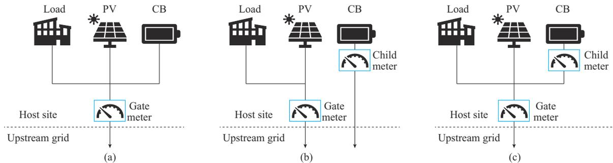
Fig. 1. Example diagram. (a) BTM architecture. (b) FOM architecture. (c) Proposed hybrid architecture.
