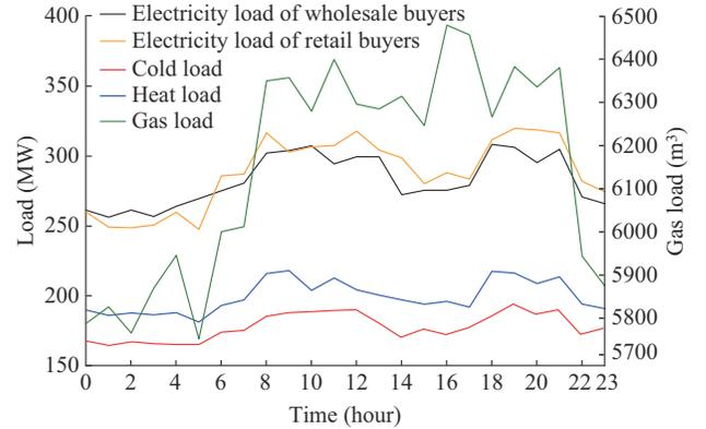
Fig. 5. Forecasted 24-hour cold, heat, electricity, and gas loads of RIES.
