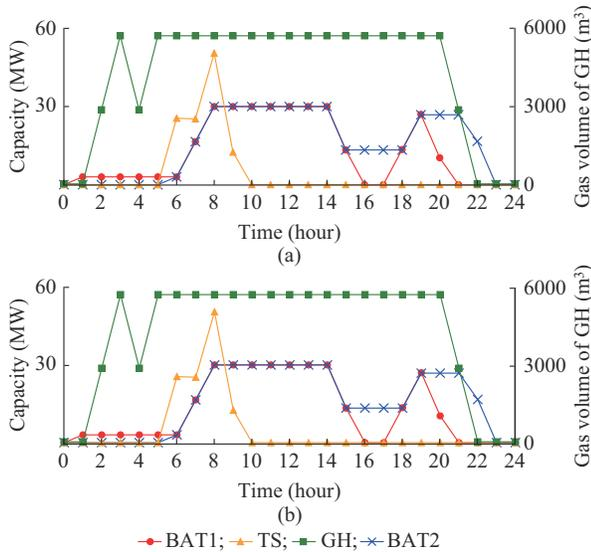
Fig. 11. Capacity of each energy storage equipment in Scheme 1. (a)  $\gamma = 0.1$ . (b)  $\gamma = 1$ .
