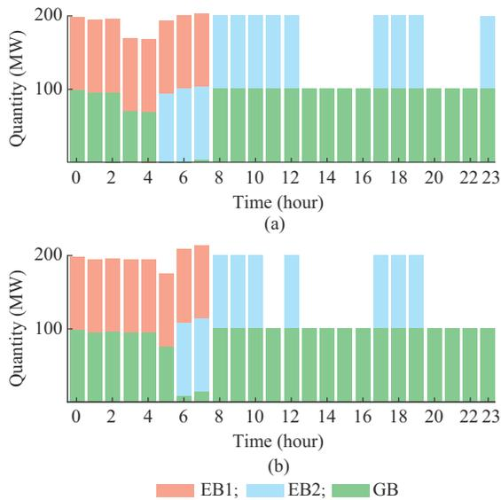
Fig. 14. Output of each heating equipment in Scheme 2. (a)  $\gamma=0.1$ . (b)  $\gamma=1$ .
