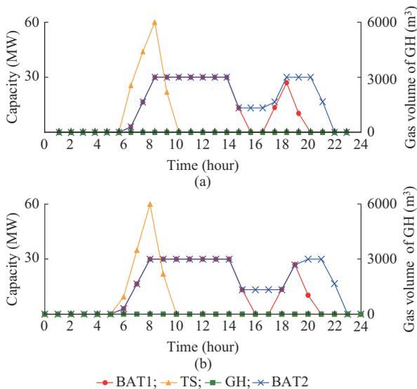
Fig. 15. Capacity of each energy storage equipment in Scheme 2. (a)  $\gamma=0.1$ . (b)  $\gamma=1$ .
