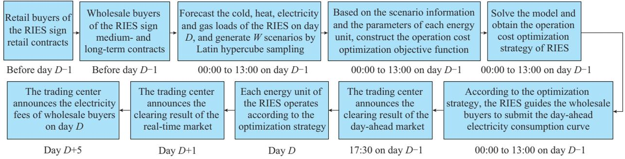
Fig. 3. Flow chart of proposed optimization method.
