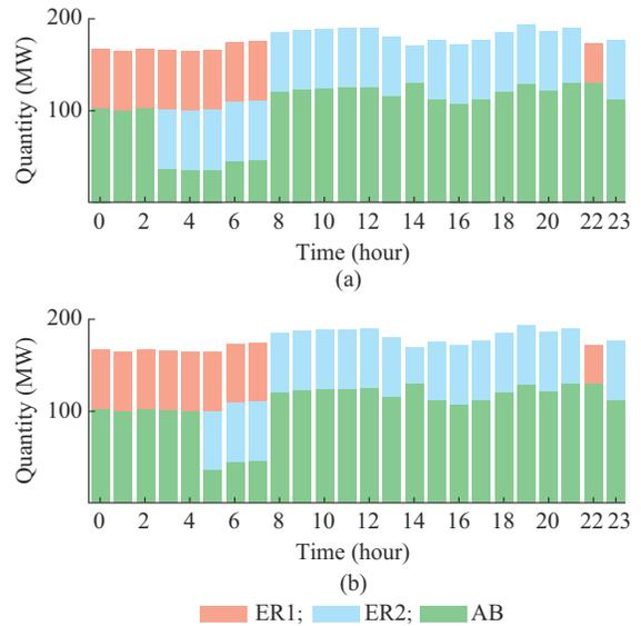
Fig. 13. Output of each refrigeration equipment in Scheme 2. (a)  $\gamma = 0.1$ . (b)  $\gamma = 1$ .
