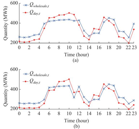
Fig. 12. Total submitted electricity quantity and actual electricity consumption in Scheme 2. (a)  $\gamma = 0.1$ . (b)  $\gamma = 1$ .
