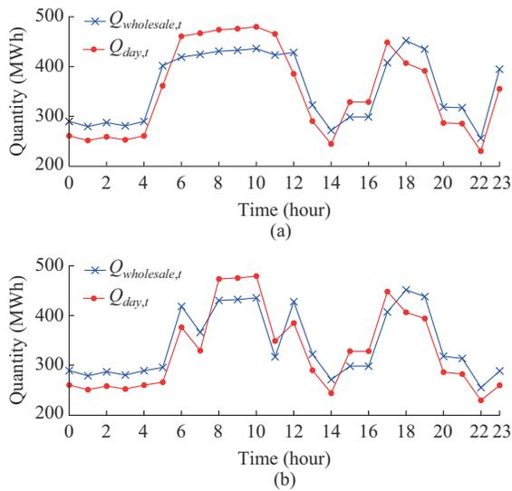
Fig. 8. Submitted electricity quantity and actual electricity consumption in Scheme 1. (a)  $\gamma=0.1$ . (b)  $\gamma=1$ .
