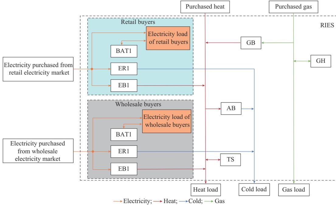
Fig. 1. Operation cost structure of RIES in electricity market environment.
