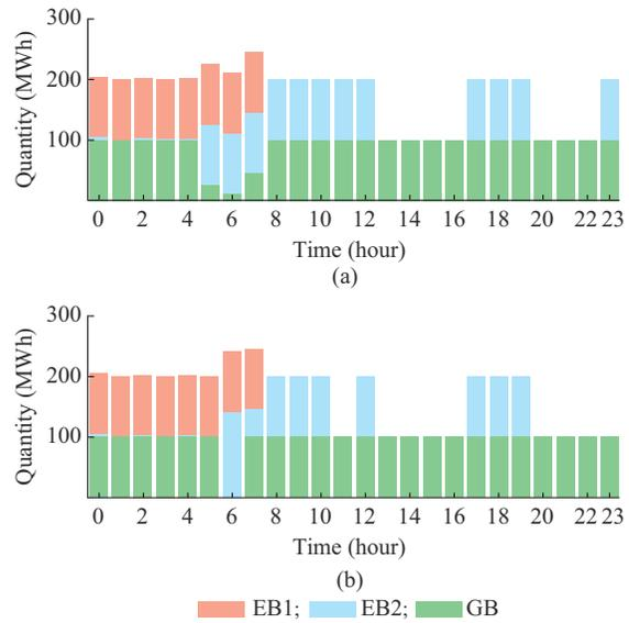
Fig. 10. Output of each heating equipment in Scheme 1. (a)  $\gamma=0.1$ . (b)  $\gamma=1$ .
