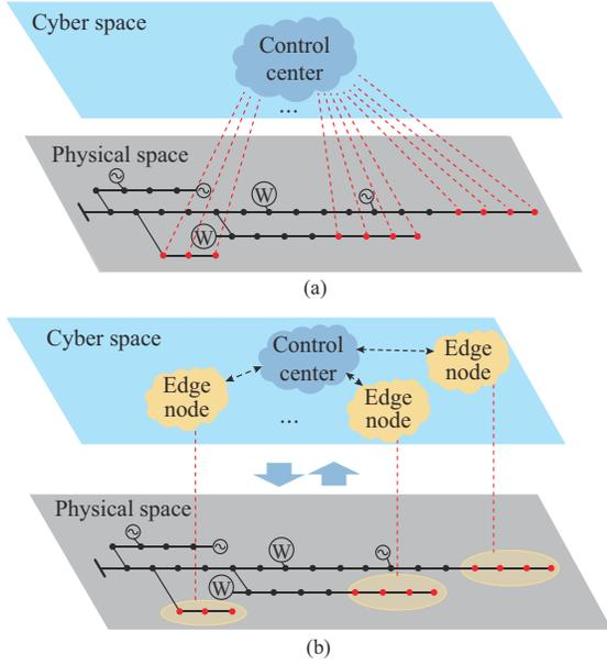
Fig. 1. Comparison of two different calculation frameworks. (a) Centralized computing paradigm. (b) Edge computing paradigm.
