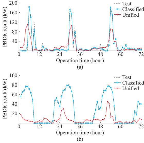
Fig. 7. Performance comparison of unified and classified XGBoost-based PBDR modeling. (a) PBDR modeling results of load node 8. (b) PBDR modeling results of load node 10.
