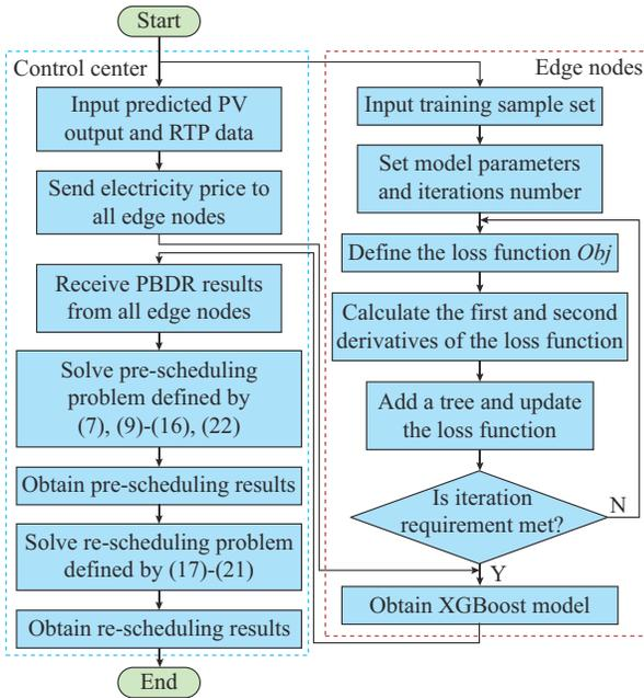
Fig. 4. Interaction process of control center and edge nodes.
