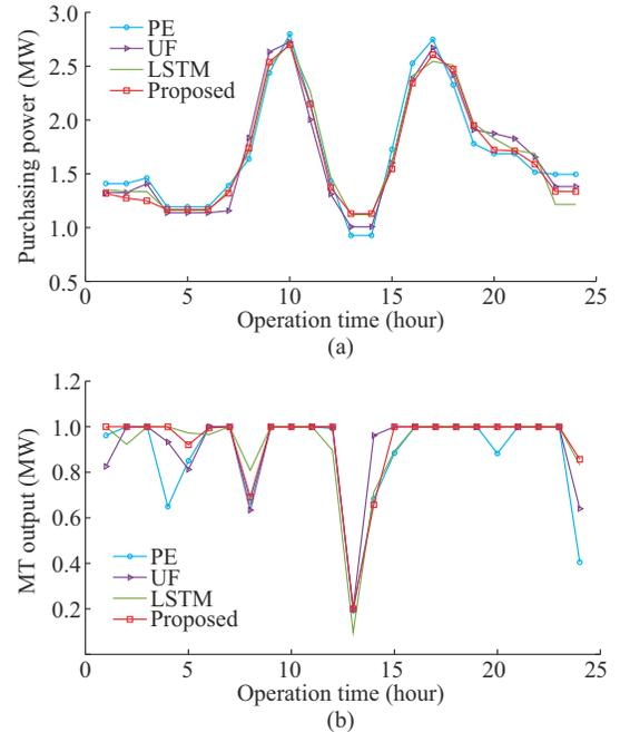
Fig. 10. Pre-scheduling results of distribution system with different PBDR modeling methods. (a) Pre-scheduling results of purchasing power. (b) Pre-scheduling results of MT output.
