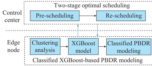
Fig. 2. Interactive optimization framework between control center and edge nodes.
