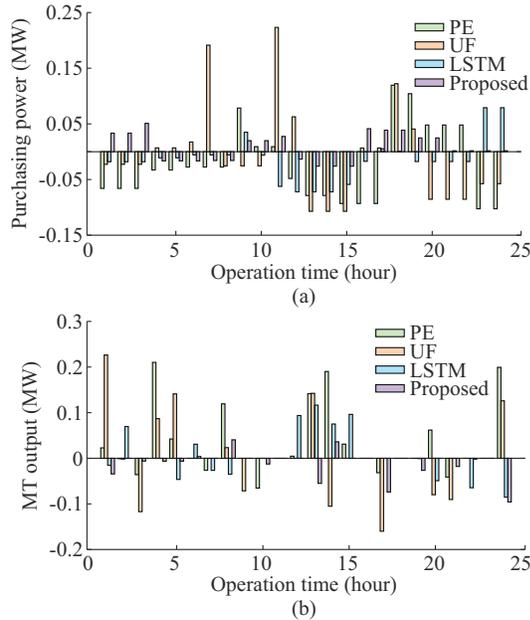
Fig. 11. Re-scheduling results of distribution system with different PBDR modeling methods. (a) Re-scheduling results of purchasing power. (b) Re-scheduling results of MT output.
