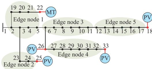
Fig. 5. Topology of modified IEEE 33-node distribution system.
