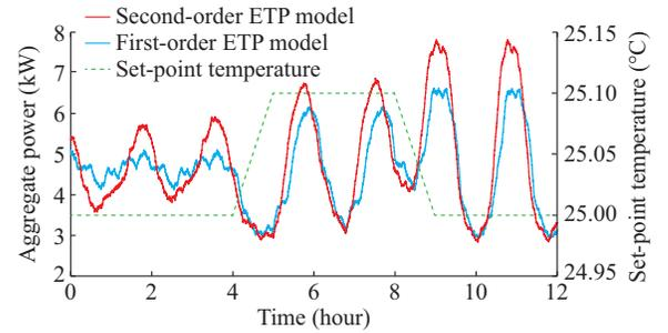
Fig. 5. Comparative results of first-order ETP model with second-order ETP model.
