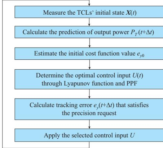
Fig. 3. Control flow chart of ILMPC.
