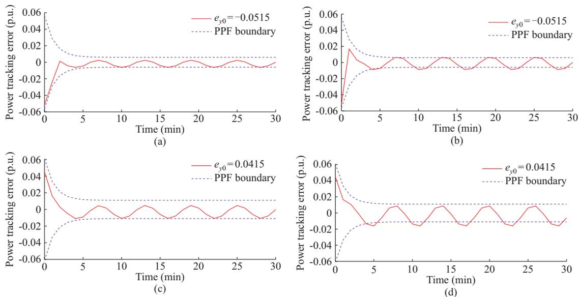
Fig. 11. Comparisons of power tracking error with different control approaches under more realistic reference power. (a) Proposed ILMPC in the first group simulation. (b) LMPC in the first group simulation. (c) Proposed ILMPC in the second group simulation. (d) LMPC in the second group simulation.
