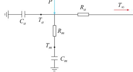
Fig. 1. Thermal equivalent circuit of second-order ETP model for individual TCL.
