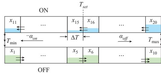
Fig. 2. Dynamic process of TCLs after finite-difference discretization.
