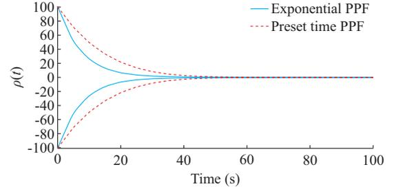
Fig. 4. Simulation results for exponential PPF and preset time PPF.
