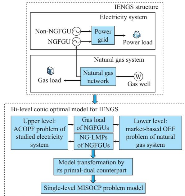
Fig. 1. Bi-level conic OEF model.
