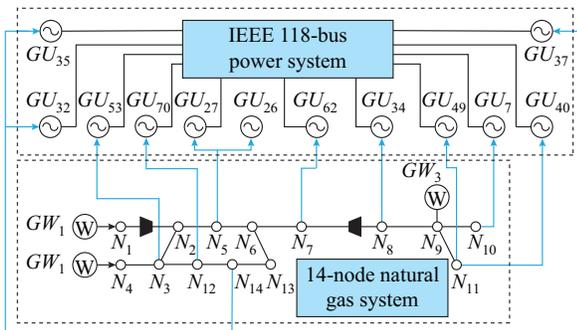
Fig. 4. Topology of IEEE 118-bus power system with 14-node gas system.
