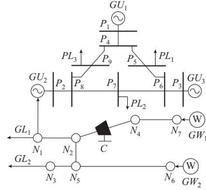
Fig. 2. Topology of IEEE 9-bus power system with 7-node gas system.
