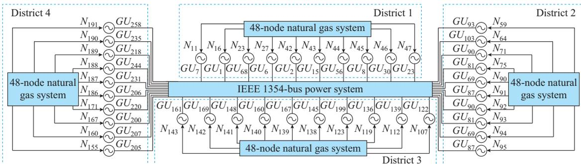
Fig. 7. Topology of IEEE 1354-bus power system with 4 × 48-node gas systems.
