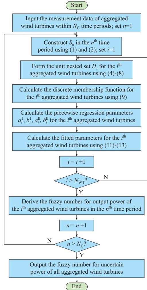
Fig. 2. Flow chart of proposed NSM.
