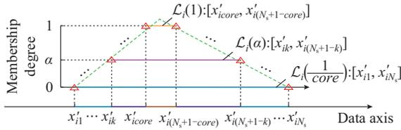
Fig. 1. Illustration for nested set and triangular shape of discrete membership function.
