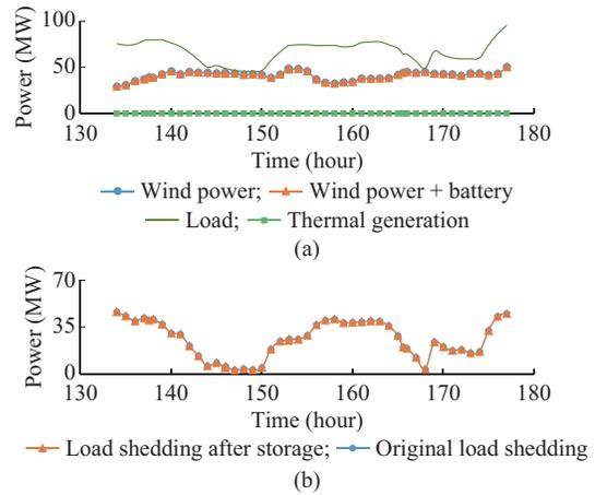
Fig. 3. Elimination of reliability worsening using operation strategy 2. (a) Power generation and system load during failure of thermal power plant. (b) Load shedding during failure of thermal power plant.
