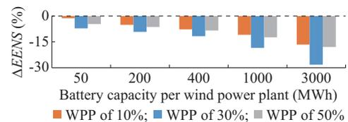
Fig. 7. Reduction of EENS index with CF of 51%.
