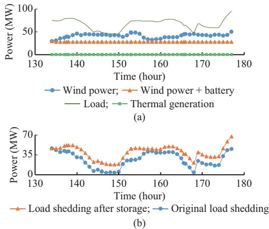
Fig. 2. Reliability worsening using operation strategy 1. (a) Power generation and system load during failure of thermal power plant. (b) Load shedding during failure of thermal power plant.
