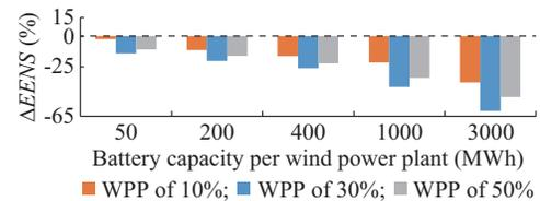
Fig. 6. Reduction of EENS index with CF of 25%.
