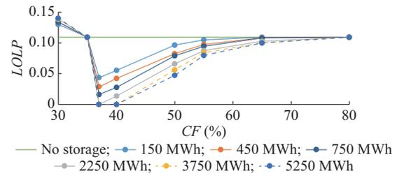
Fig. 1. Variation of LOLP with CF and storage capacity.
