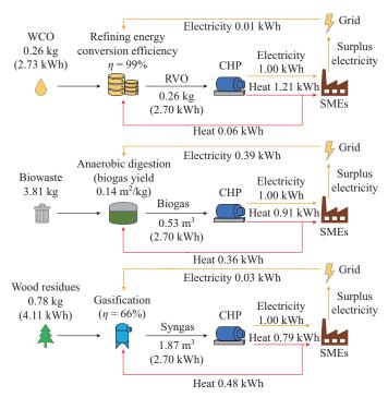
Fig. 1. Graphic scheme of systems under evaluation.
